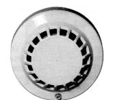
The IR3-M1 is a fire smoke detector for the LOOP 500 and MTG systems. It corresponds to DIN EN 54-7 for fixed-point detectors. It responds to various invisible smoke gases (aerosols) and visible smoke. It is use in a fire alarm system does not require a licence. It is equipped with an automatic test chamber monitor, which sends a signal via the primary loop to the control panel if the test chamber in the LOOP 500 system becomes contaminated or develops a fault.
